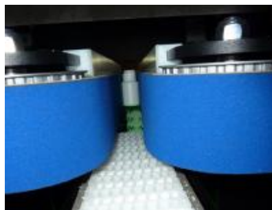
- (2) camera top and bottom inspection
